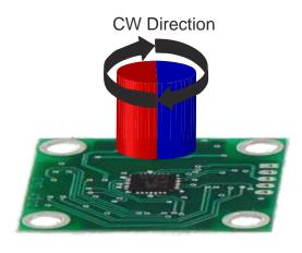
MDB28 magnetic rotary encoder module has a precision sensor having an integrated Hall element for scanning a permanent Dipole magnet. The Sensor itself generates a constant amplitude Sine and Cosine voltages that is used for angle calculations. These Sine and Cosine signals are further interpolated to get the Incremental or Absolute signals with resolutions up to 14 bits per rotation.
