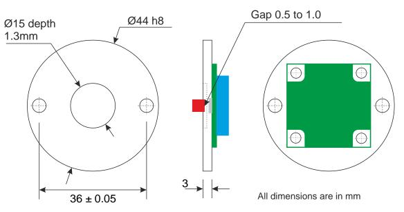
**Note:** Magnet center axis and PCB center should be with in ± 0.2mm to get the specified accuracy results
