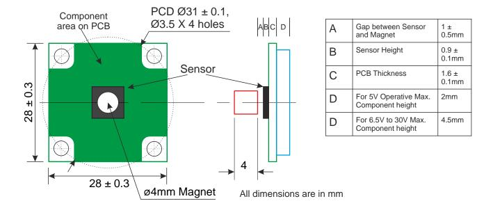
**Note:** Magnet center axis and PCB center should be with in ± 0.2mm to get the specified accuracy results
