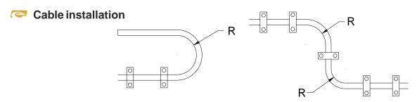
**Note:** Minimum possible R is 25mm Tested at 500000 strokes at minimum bending radius
