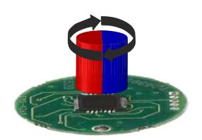
MDE16 is a very compact magnetic rotary enclosed encoder with a shaft. It has a precision sensor having an integrated Hall element for scanning a permanent Dipole magnet. The encoder can give Absolute as well as incremental outputs up to 14 bits per rotation.
